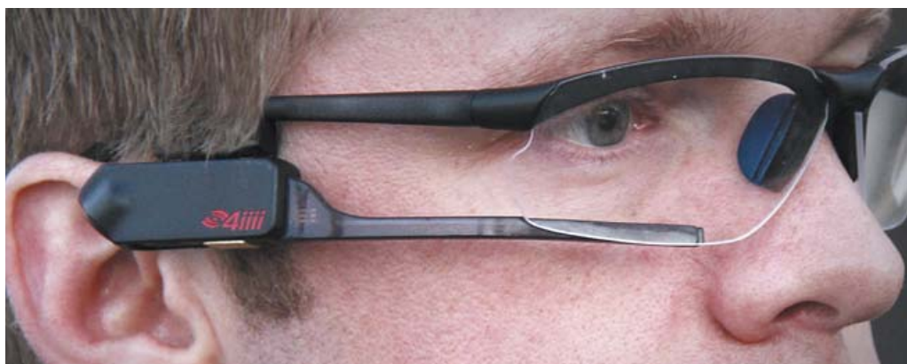
4iiii's Sport-iii's uses ANT wireless technology to inform fitness enthusiasts of how they're performing via a head-up display.
