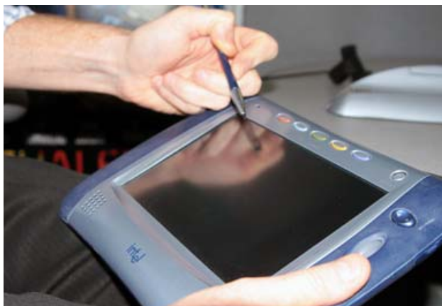
The Intel Web Tablet utilized a touch screen design or a stylus for navigation.
